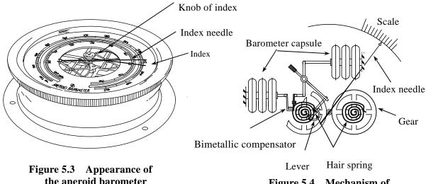
Figure 5.4 Mechanism of the aneroid barometer
