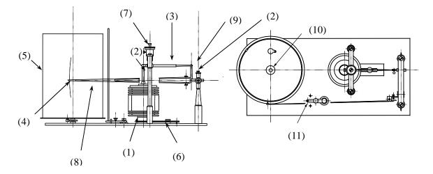
Figure 5.5 Structure of the aneroid barograph
