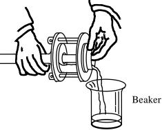
Figure 5.14 Pouring mercury into a beaker
