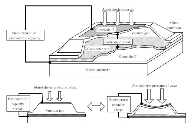
Figure 5.8 Pressure sensor of the electrostatic capacity barometer
