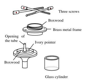
Figure 5.16 Parts of mercury cistern glass cylinder
